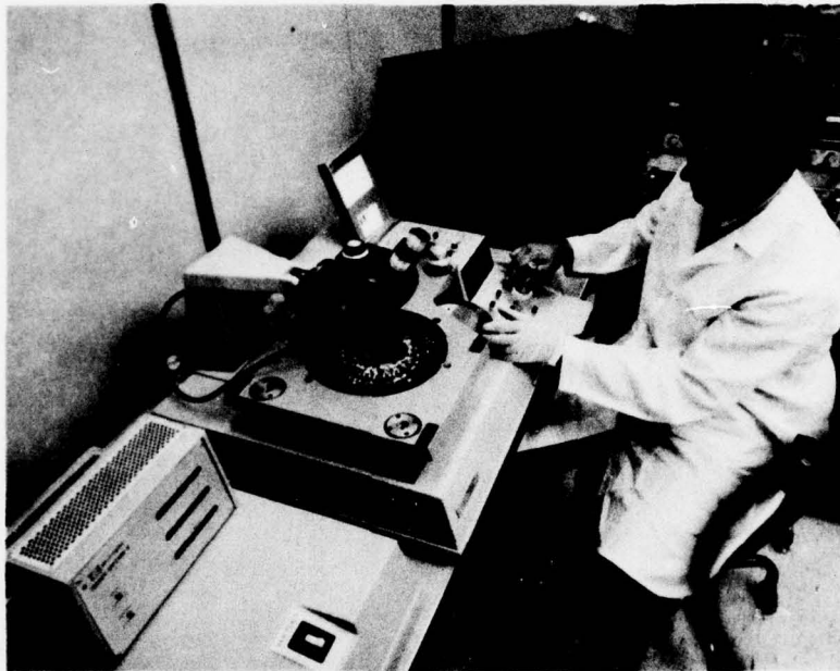
Fig (13) The automatic circuit test facility- probe station
